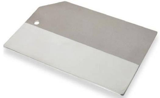
The daily System Performance Check involves running the test panel through the production penetrant system and examining the results. The appearance, number of indications, and quality of indications are compared to the baseline established for each test panel and each system. Any change should be investigated and corrected. It is recommended that each Known Defect Standard be "re-calibrated" or baseline at least once per year and after significant changes to the penetrant system.
